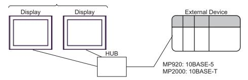
\*2 When Ethernet port on CPU unit in MP2310/MP2300S/MP2400 is used, up to 4 Displays can be connected.
